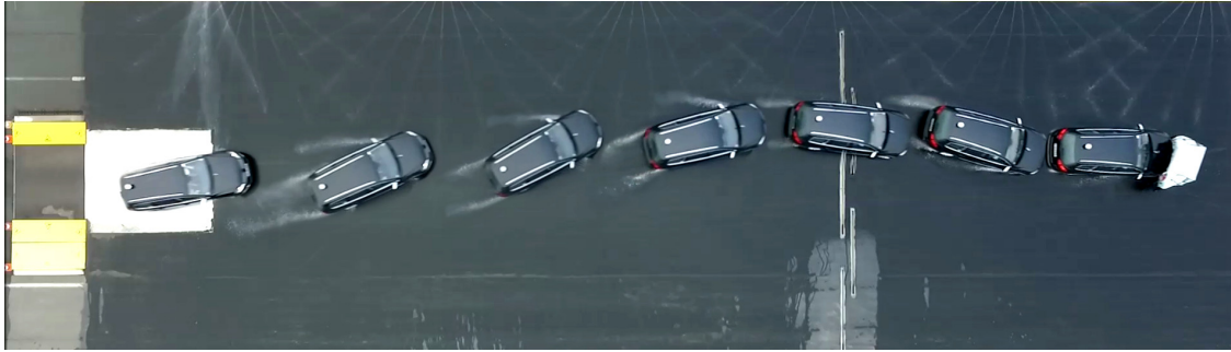
Figure 4.1: Sequence of a dynamic test run taken with a drone; time step: 0.5 s [KHD + 17] © 2017 IEEE.
